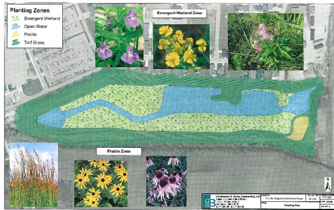
"Wetland plantings at F-Lake Regional (stormwater quantity (detention) and quality control) Basin, Lafayette, IN" used by permission of the Tippecanoe County Surveyor's Office.
